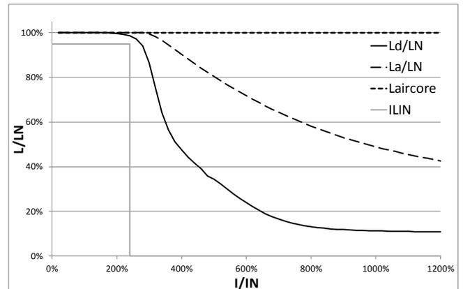
**Figure 3: Computed Linearity of Iron-Core Reactor**
