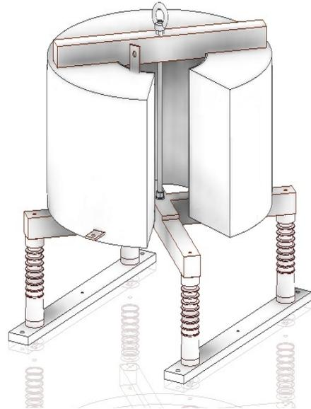
Figure 1: Air-Core Reactor on Post Insulators
