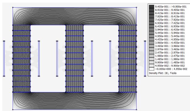
Figure 4: Magnetic Field of an Iron-Core Reactor
