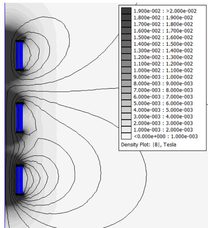
Figure 5: Magnetic Field of an Air-Core Reactor in Top-On-Top Design (only one half shown due to axis symmetry)
