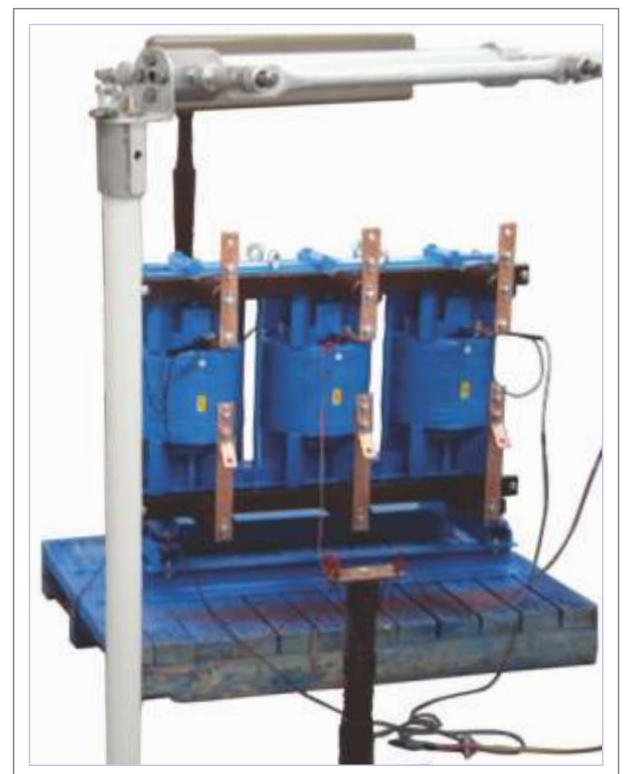
BIL test on MV Iron Core Reactor
